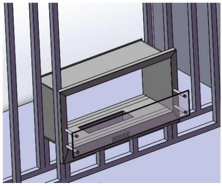
5. Install a stud horizontally on top of the firebox to be able to continue with the wall.
