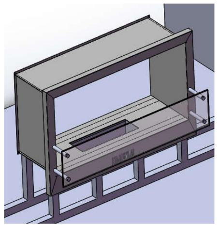
3. Continue building the wall, ensuring that there is a layer of cement board between the stud and your Firebox on all sides.
