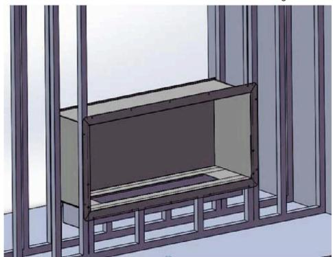
5. Install a stud horizontally on top of the firebox to be able to continue with the wall 6.Screw the top of horizontal stud directly to the Firebox brackets (use 0.5 inch metal zips)
